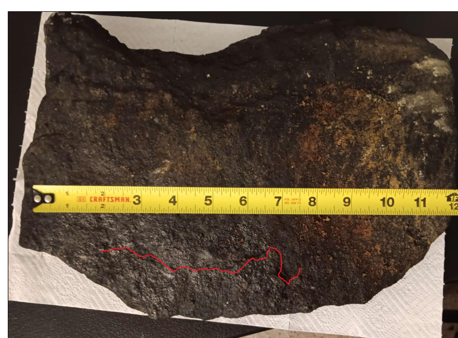
Figure 6) The crack that appeared in the rock, underlined in red for clarity
