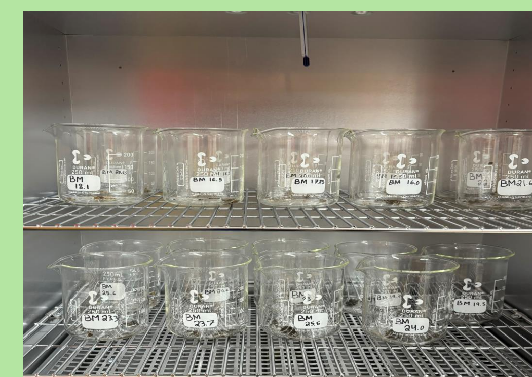
The 2-g samples were then rinsed in DI water, the clean samples were then dehydrated in lab oven.
