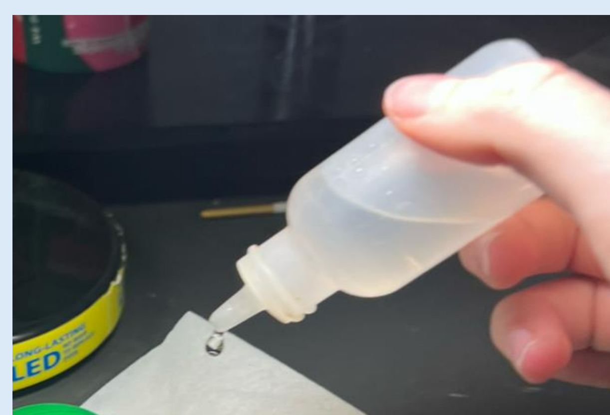
Test sample from the Jefferson formation with HCl to determine lithology; Dolomite or Calcite, and log in Excel.
