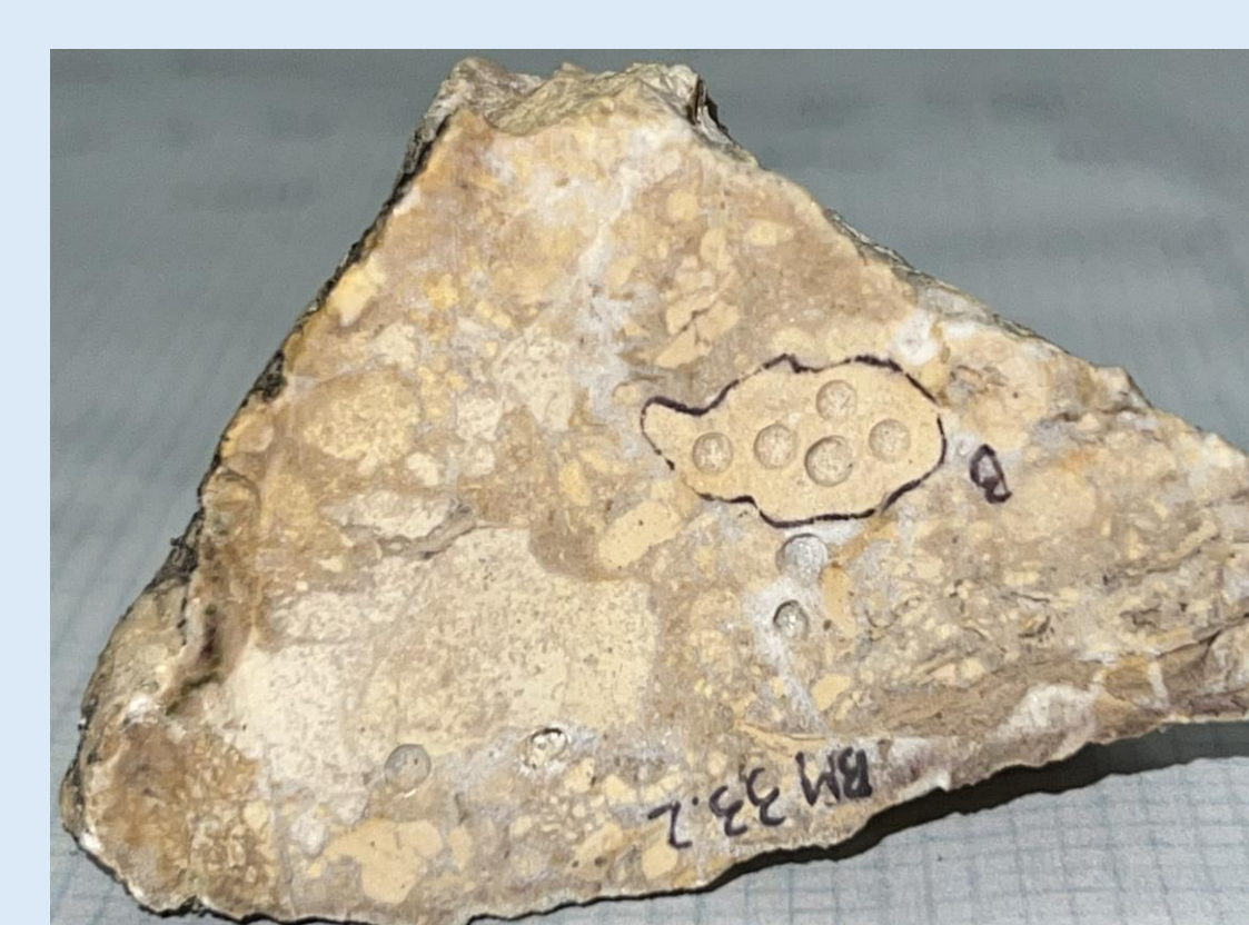
Drill Jefferson sample in area of interest to obtain ~1ml of powder for testing.
