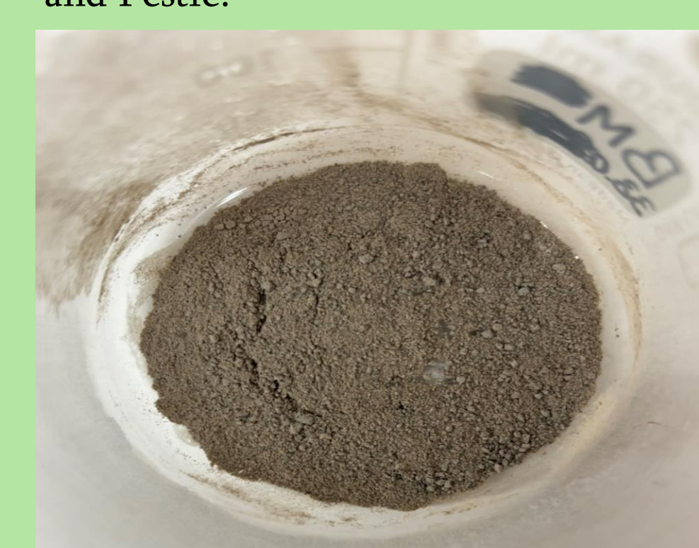
Powdered samples were then transported into a labeled beaker to be acidified by HCl solution.
