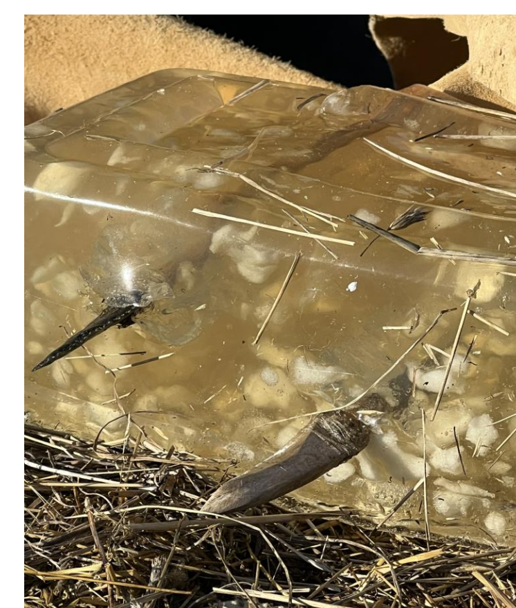
Figure 5. First round of testing, showing the exit wounds on the gel.
