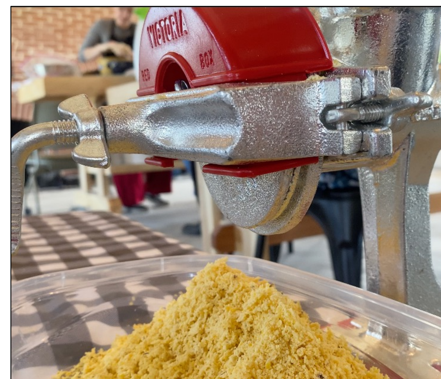
Figure 4: After nixtamalization, the corn is ground to a fine grain using a hand-cranked grinder
